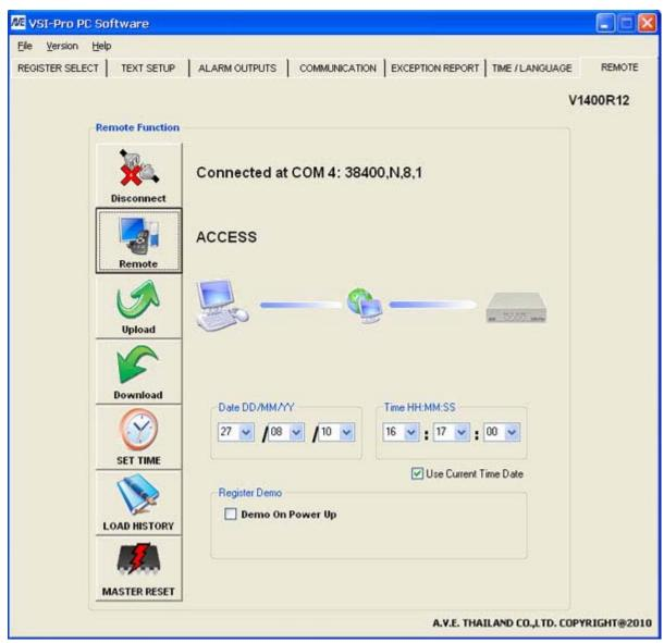
Figure 71B: VSI-Pro PC Software can establish communication with VSI-Pro Max 8
