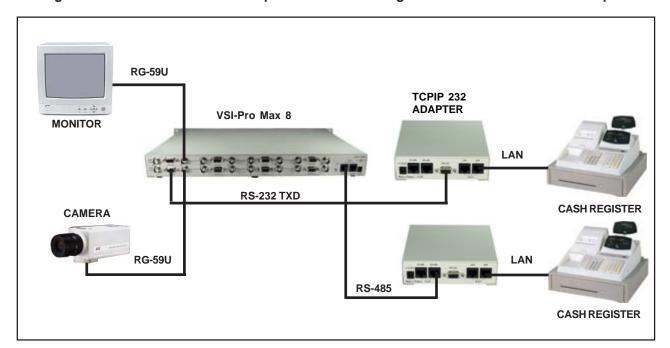
Figure 144: VSI-Pro Max 8 Connections with TCPIP 232 Adapter
