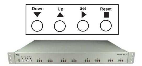
Figure 5: Four Front Pannel Push Buttons of VSI-Pro Max 8
