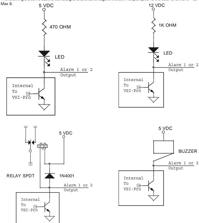
Figure 112: Hard Alarm Output
