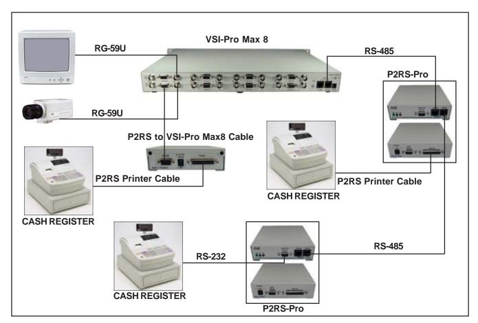
Figure 127: VSI-Pro Max 8 with P2RS and P2RS-Pro Connections
