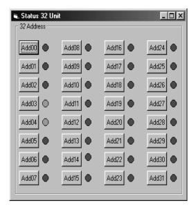
The **Green** Led is indicated when a Networker is Detected. The **Red** Led is indicated no Networker at that Address.
