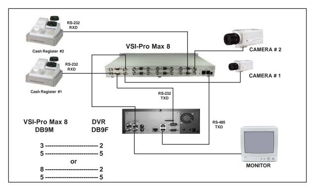
Figure 113: VSI-Pro Max 8 with DVR Text Input Connections
