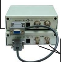
Use the BNC connectors of the VSIB for your Video Input & Output The pin-out for the VSIB between the VSI-Pro and the VSIB is as follows:
