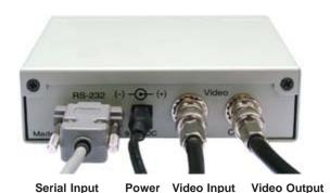
Figure 133: VSIB Connection Cables
