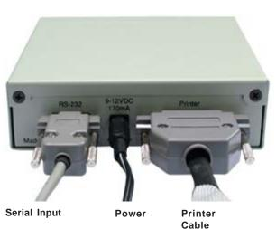
Figure 121: P2RS Parallel-to-Serial Converter Connection Diagram
