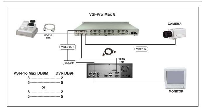
Figure 80: VSI-Pro Max 8 with DVR Control Connections
