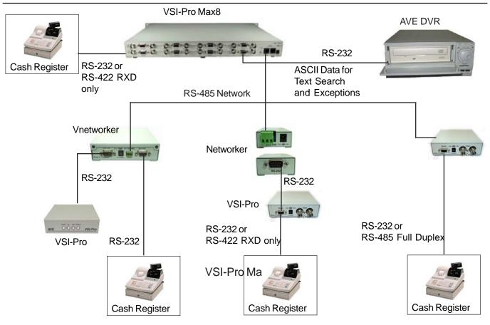
Figure 152: VSI-Pro Max8 Vnetworker Connection
