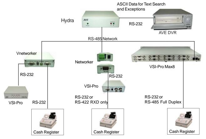
Figure 153: Hydra Vnetworker Connection
