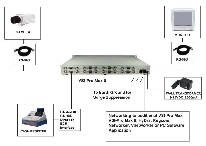
Figure 3: VSI-Pro Max 8 Connections
